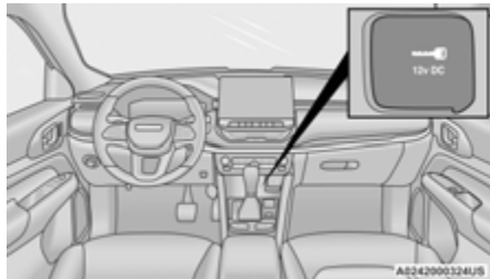
Front Power Outlet
