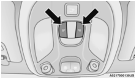
Overhead Light Switches
