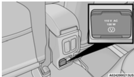
Power Inverter Location
