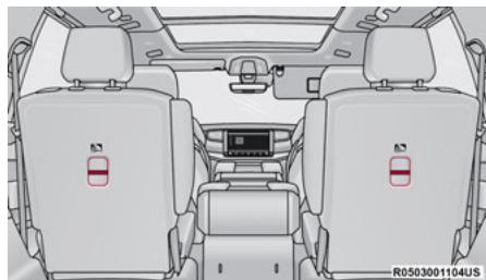
Seven Passenger Top Tether Anchorages (Captain's Chairs)
